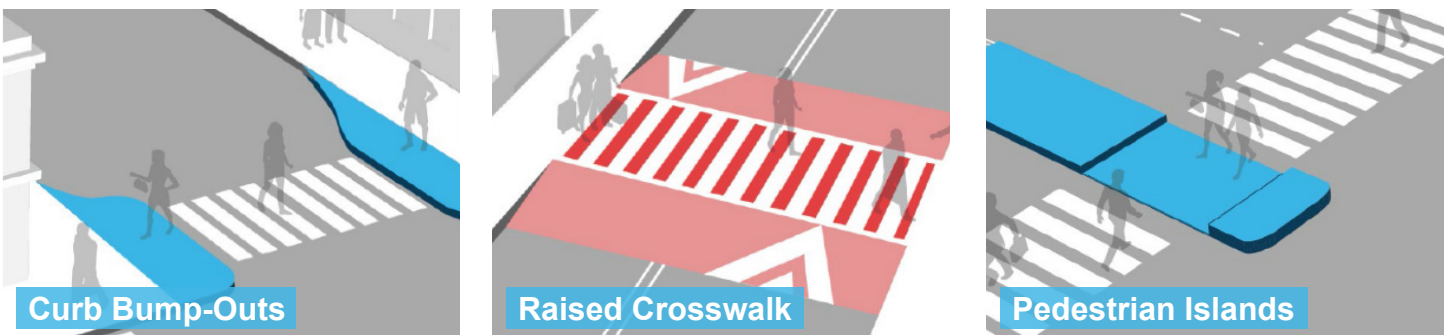
Figure 2. Potential access and safety improvements
